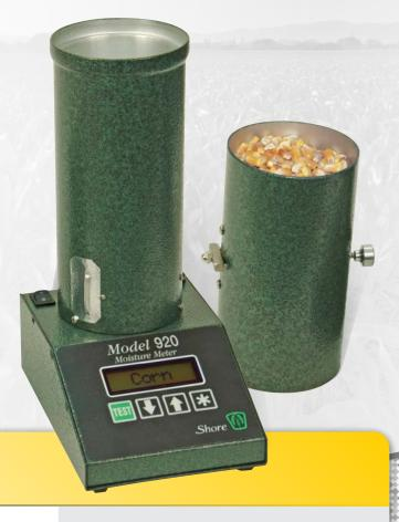
The Shore Model 920 Moisture Tester offers quick, accurate testing for a large variety of commodities. Utilizing proven cell design and measurement principles, the Model 920 delivers results that closely match meters used by grain elevators. This means you can confidently measure moisture content before going to market.
